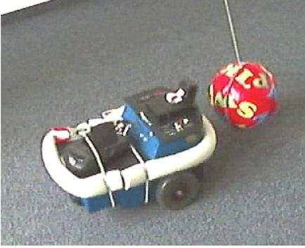
Figure 5: Typical situation of the Pioneer robot in visual contact with a ball. The controller initially is in the tabula rasa condition. Over a time of several minutes the robot gradually begins to move, to develop a sensorial contact and later on to react sensitive to the movements of the ball. In this initial phase the ball is suspended. After some time the robot is also able to follow the freely moving ball.
