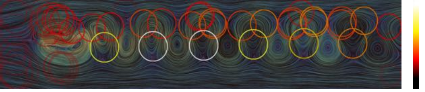
Fig. 16. For comparison, the similarity to the saddle vortex combination was laid over the LIC of the flow field with removed mean flow.
