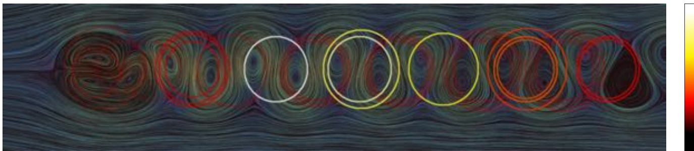
Fig. 18. The similarity of the underlying field to the counter oriented double vortex is encoded in the brightness of the circles.
