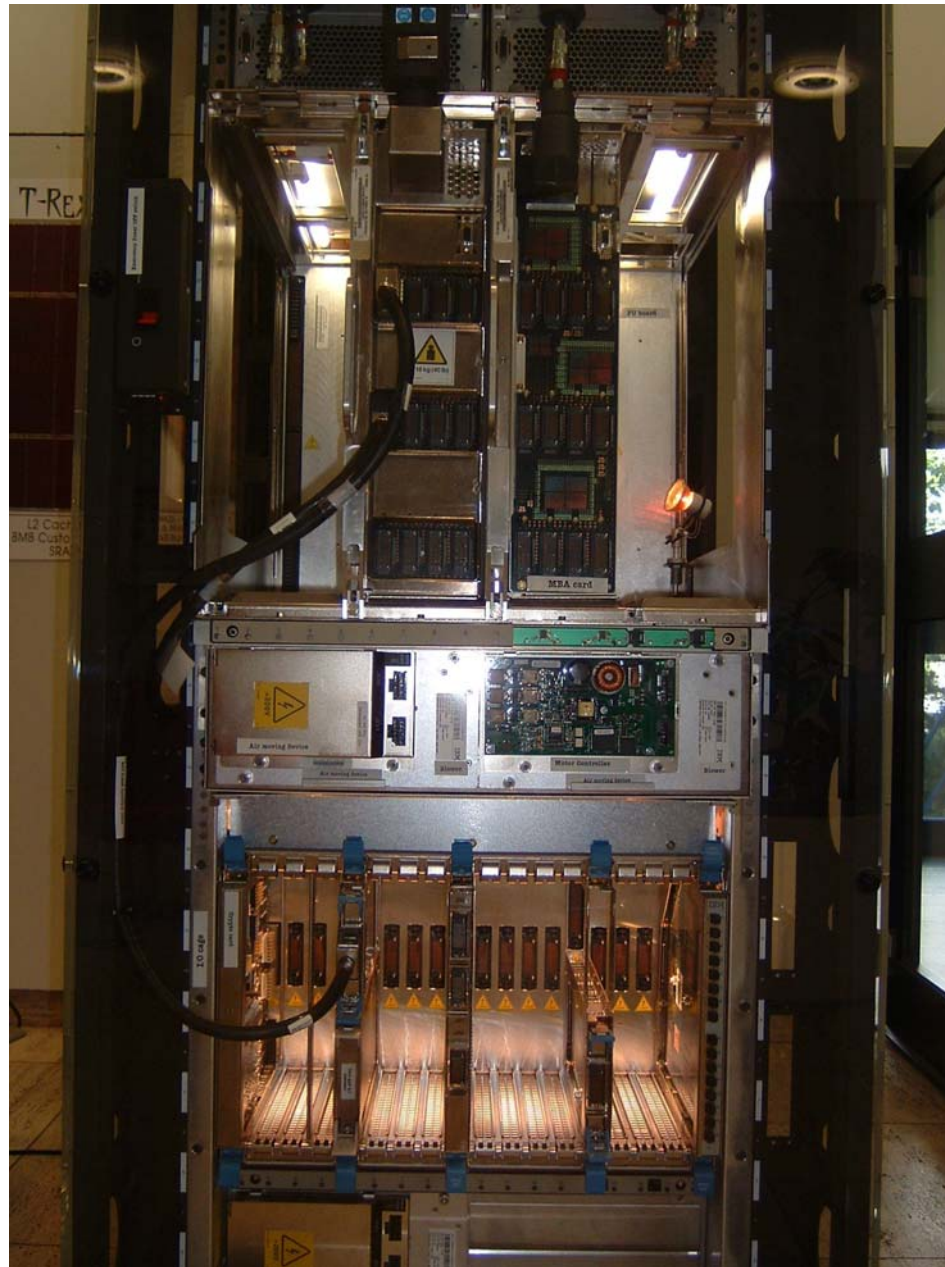
STI cable connection ton an I/O cage
