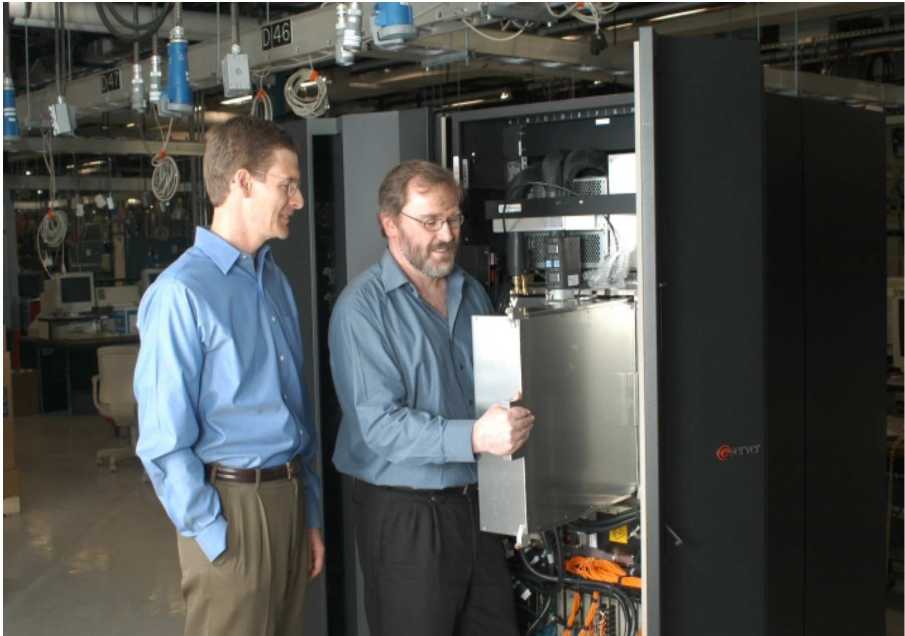
Shown is an engineer removing a book from a z9 system.
