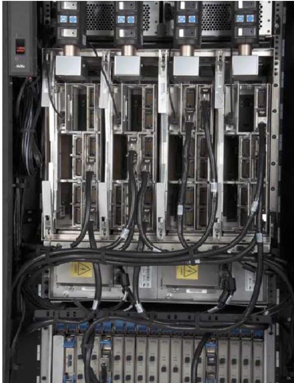
A fully populated CEC with 4 books and cables connecting to a fully populated I/O cage.
