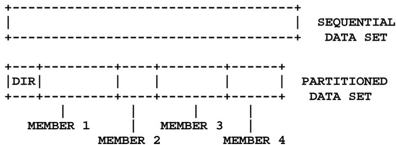
Figure 2. A Sequential Data Set and a Partitioned Data Set
