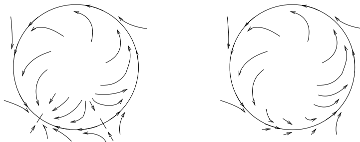
Figure 5.10: Saddle-node bifurcation on a stable cycle. The size of the arrows gives an impression (in particular in the subfigure on the right) of the flow velocity which is low near the position where the fixed points were located.
