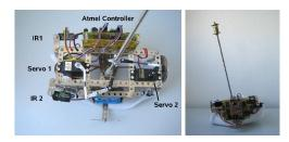
Fig. 1. Pole driven stumper. Left: close view from the top; Centre: pole to the back, Right: pole to the front
