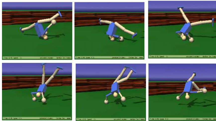
Fig. 4. The humanoid robot in a kind of back flip. The motion is from left to right and starts from a resting position (on the back) by a rapid swing of the left leg (not depicted).
