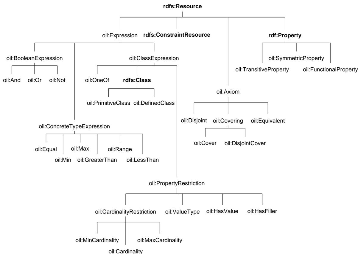
Figure 3: The OIL extensions to RDFS in the subsumption hierarchy.
